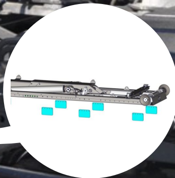
UNDERFRAME PIERCED LONGITUDINAL MEMBERS
